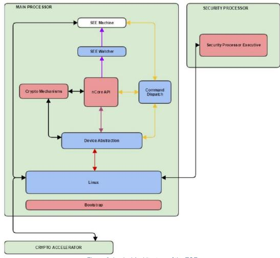
Figure 3: Logical Architecture of the TOE
