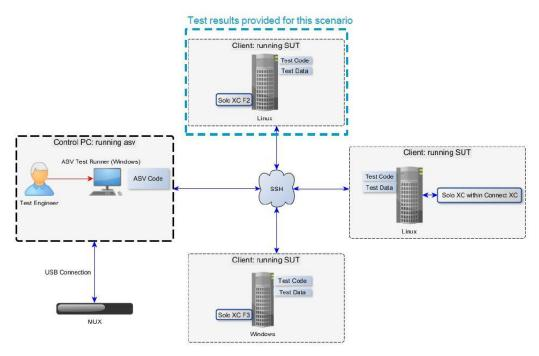
Figure 4: Developer's Test Setup
